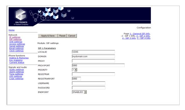
Note that the Proxy address could also be that of a peer-to-peer entity, allowing the unit to make a direct peer-to-peer to connection. This can provide an extra level of resilience, allowing the unit to fall back to a peer to peer call in the event that all proxy servers become unavailable.
