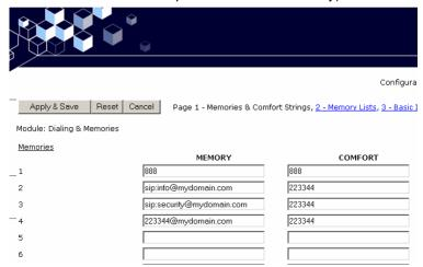
Note that comfort strings have been set to give the user confidence that "dialling" is taking place when the button is pressed.
